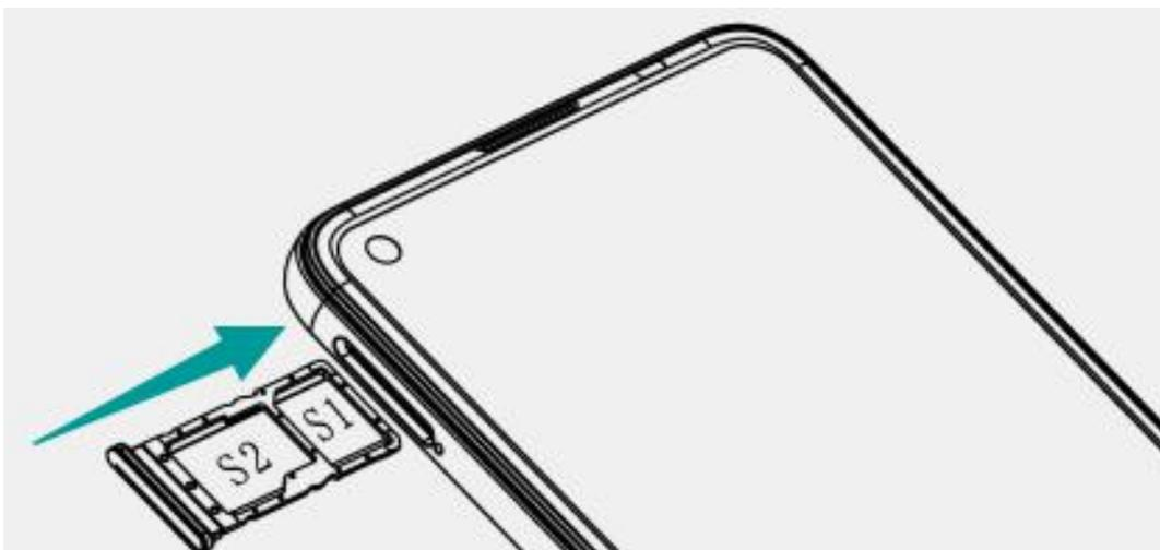
When inserting your card tray, make sure that the card is level and that the card is aligned correctly.
