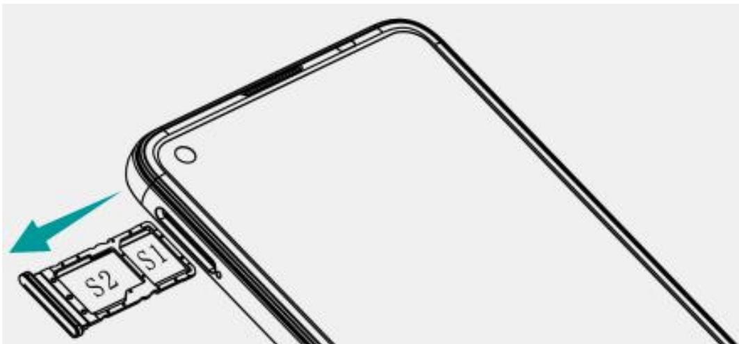
To eject SIM or MicroSD card, insert your SIM eject pin into the small hole next to the card tray.
