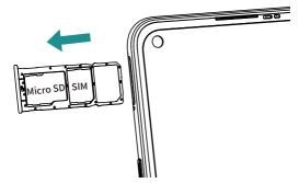
To eject SIM or MicroSD cards, insert your SIM eject pin into the small hole next to the card tray.
