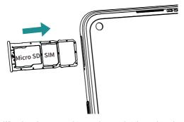
When inserting your card tray, make sure that the card tray is level and that the card is aligned correctly.
