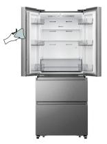
Although this appliance automatically defrosts, a layer of frost may occur on the freezer compartment's interior walls if the freezer door is opened frequently or kept open too long. If the frost is too thick, choose a time when the freezer is nearly empty and proceed as follows:
