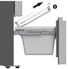
3. Remove the screws (10) fixed on the slide guides with a Philips (+) screw driver, and then remove the freezer drawer (11) by lifting it up.
