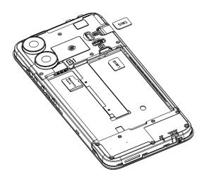
Insert the SIM card, please make sure that the direction of the SIM card is consistent with the direction on the card slot.
